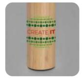
Circular UV is identical to the UV process, but optimized for 360° printing.
