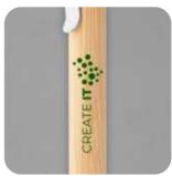
Rotary screen printing is similar to the process of screen printing, but optimized for 360° printing. This process is indicated for pens.
